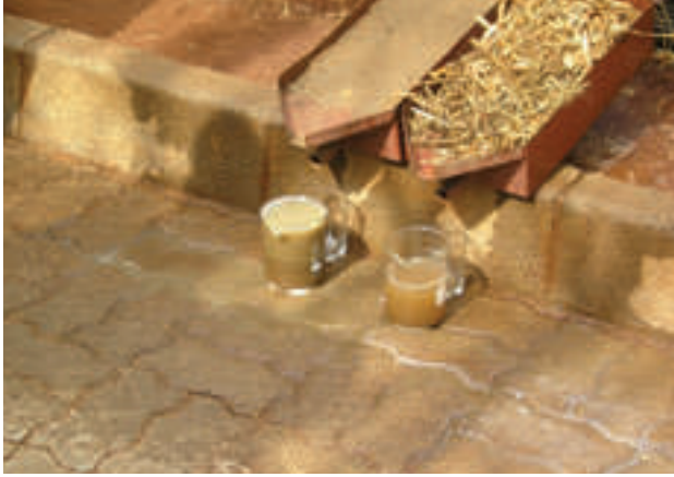
This equipment can be used to demonstrate the importance of mulch in controlling run-off and direct raindrop impact on soil erosion.
